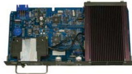
Capio Plus Dual 2400 Watt Dimming Module using IGBT Technology
