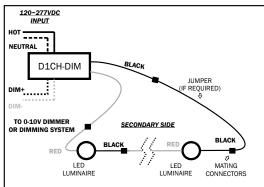
D10W-DIM-120 LED DRIVER SUPPORTS ONE TO THREE (1~3) 515 SERIES LED
