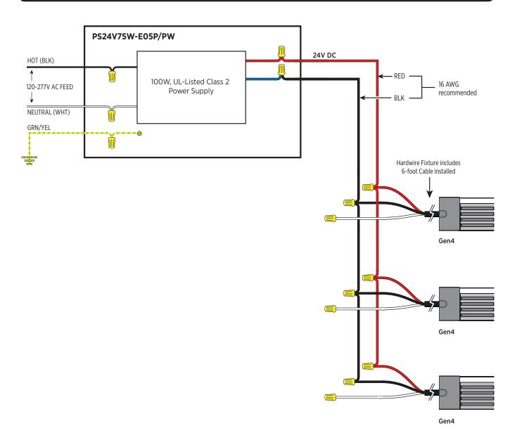
**Note:** For non-dimming installations, you should cut and cap each white wire using best industry practices.
