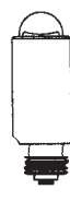
48 Grooves Per Inch 3.5V .72A 20 Hour Life Nickel Plated Xenon Filled TL-1 1/2 Lamp
