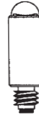
8-32 UNC Thread 3.5V .70A 20 Hour Life Nickel Plated Xenon Filled TL-1 1/2 Lamp
