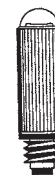
8-32 UNC 2A Thread 2.5V .30A 15 Hour Life Nickel Plated Vacuum TL-1 1/4 Lamp
