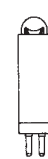
0.55mm Leads=CL1419 0.80mm Leads=CL 1421 3.5V .74A 40 Hour Life Nickel Plated Krypton Filled TL-1 1/2 Lamp
