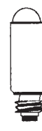
10-32 UNF 2A Thread 2.5V .68A 20 Hour Life Nickel Plated Xenon Filled TL-1 1/2 Lamp
